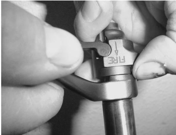
Disassembling the bolt can be done in the field, but remember, there are small parts involved, some of which are under spring tension.
