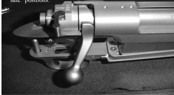
3. Push the bolt fully forward, positioning a new cartridge from the magazine into the chamber. Lock the bolt by moving the bolt handle (knob) fully down. Your rifle is again cocked and ready to fire. Immediately put the safety in the middle or rear “on safe” positions until you are ready to fire again (see Figure 16).
